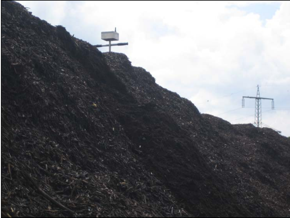
Figure 6 Measuring probe “NaviRott®” in a windrow of bulking material and pre-treated organic waste
