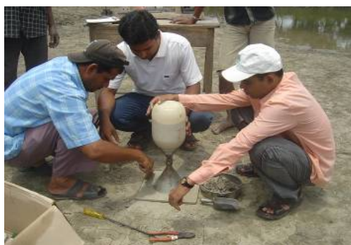
Figure 11 Field density test of the CCL
