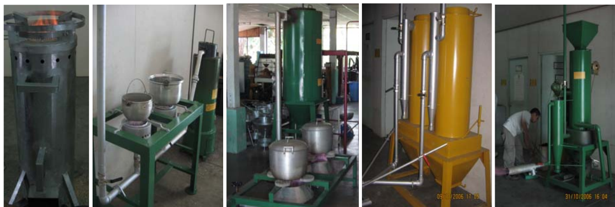
Figure 3 Gasifier technologies designed for biomass waste utilization, namely from left to right: single-burner, multi-burner, dual-reactor, and continuous-flow type gasifiers
