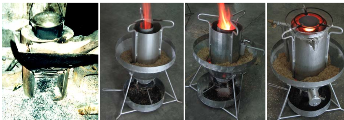
Figure 2 Direct combustion stoves developed for biomass waste utilization, namely from left to right: step-grate stove, conical stove, side-in, and the super turbo
