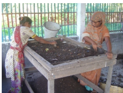
(a) Wooden frame screening system
