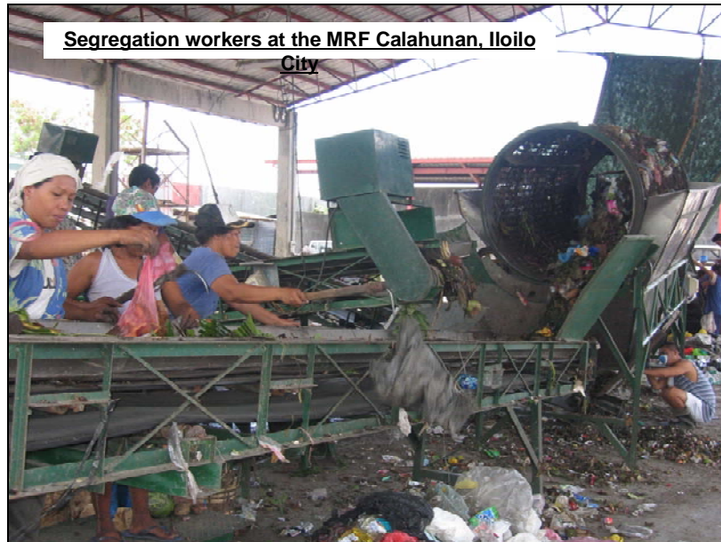
Figure 3 Waste workers segregate materials which passed the trommel screen at Calahunan MRF
