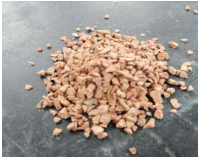
Figure 1 Picture of wasted roof tile
