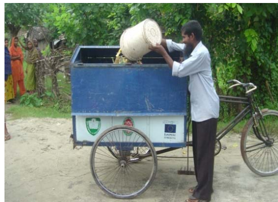
Figure 2 Newly designed manually driven Rickshaw Van for door-to-door collection
