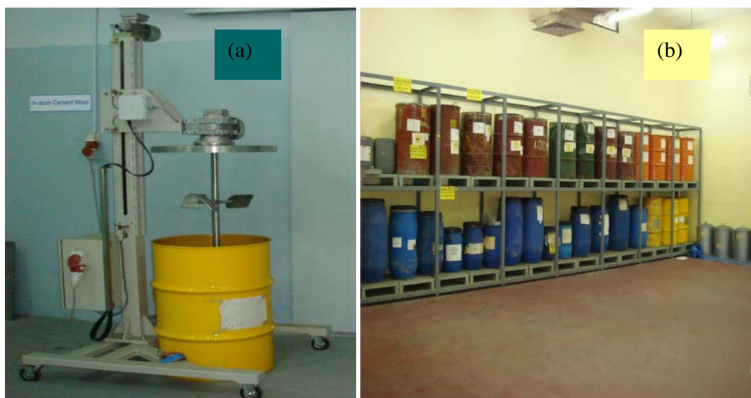
Figure 3 (a) In-drum cement mixer for solid waste conditioning and (b) Interim-storage (solid RWs)
