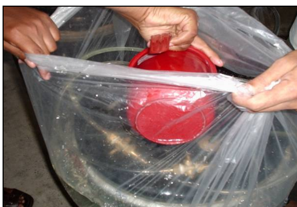
Figure 3 Checking up of leakage
