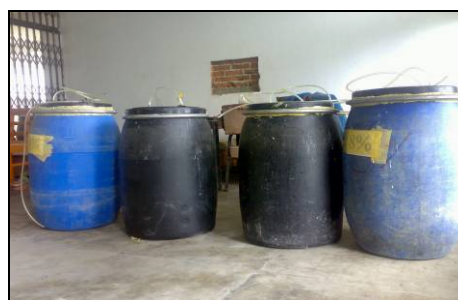
Figure 2 Drums for anaerobic digestion
